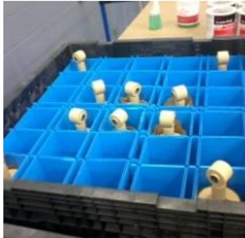
AIM Reusable Packaging designed this pack to eliminate waste spending on expendable packaging. (60) 48"x45"x42" plastic knockdown bulk bins with (60) plastic corrugated packs to hold (30) parts per bin , part weight 69 lbs. These packs are currently being shipped from Canada to Wisconsin.
