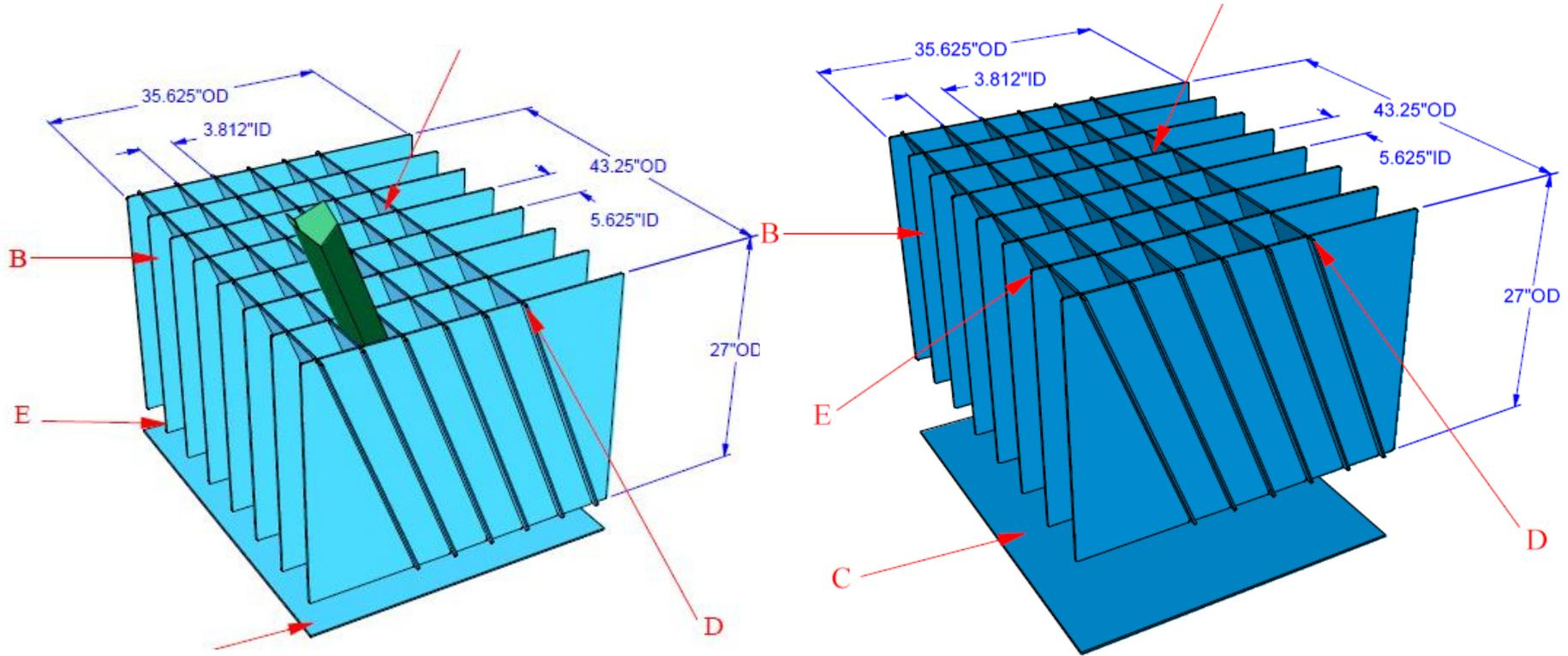
AIM Reusable Packaging designed this pack to protect and divide the Plenum Side Chamber. In the process the plastic corrugated pack will save money as opposed to paper corrugated they had been using. Currently using (30) partitions introduced into a 48"x40"x34" tall plastic bulk bin.
